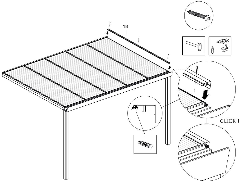
12. Now screw a sheet stopper at the gutter end of each middle beam to ensure secure attachment.
