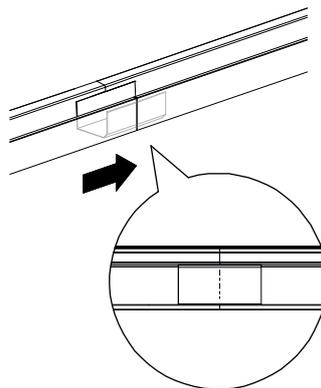
**5.** Now press the second gutter completely over the gutter extension to form a seamless joint.
