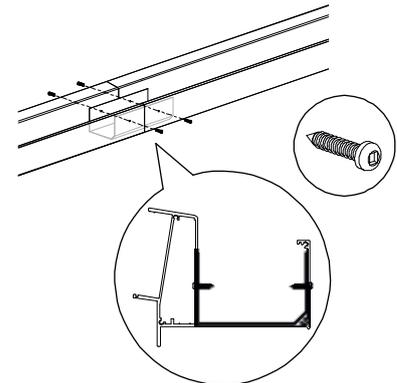
**6.** The gutter connector can now be secured with the short stainless steel screws in the chamber of the gutter and on the front side under the decorative profile. Apply sealant on the assembly so it is smooth and waterproof!
