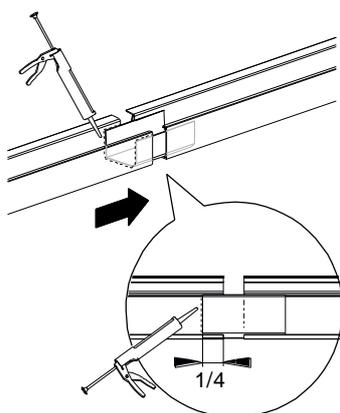
**4.** Insert the second gutter  $\frac{1}{4}$  of the way into the other side of the extension and apply sealant on the edge.
