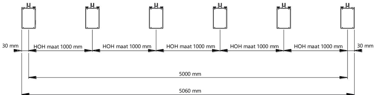
When standard size sheets are used, the total width of joined roofs must therefore also end with 60 mm, e.g. 8060, 9060, 10060, etc.
